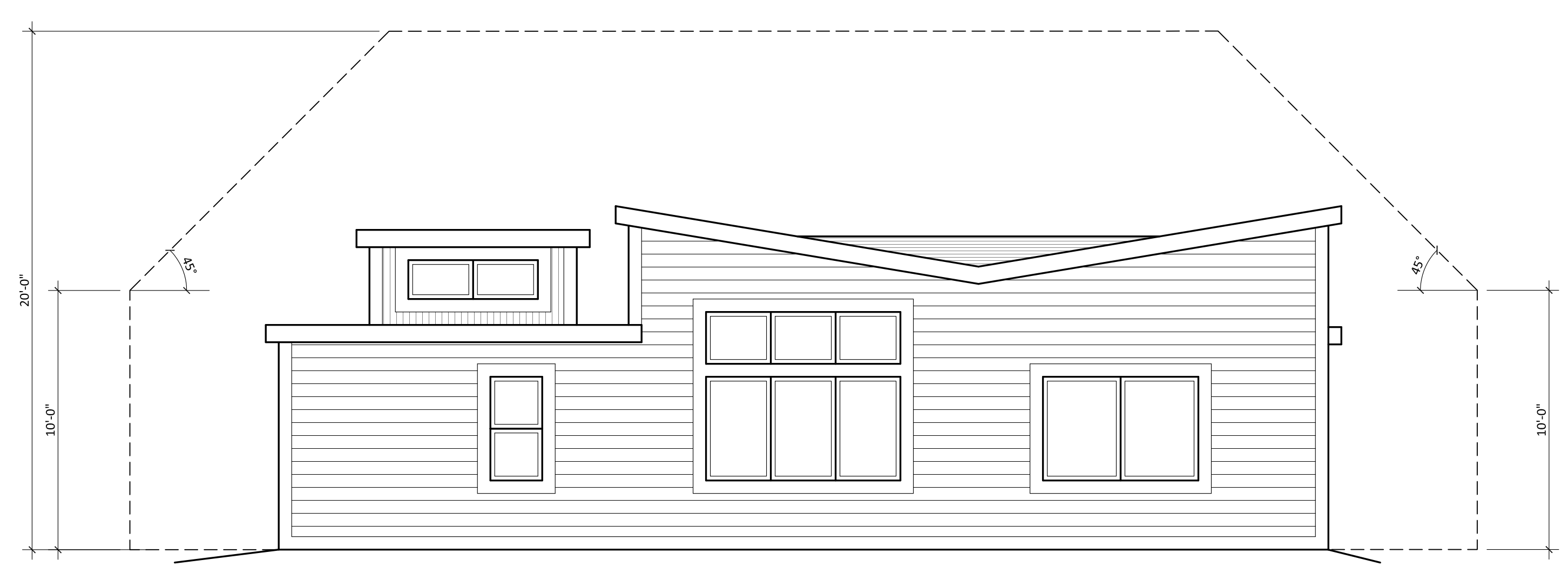
EXTERIOR ELEVATION - REAR (TYPE-2)
